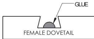
FIG#1 - CABINET PART GLUE APPLICATION
